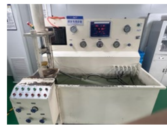
Pressure Test for Large Valve
