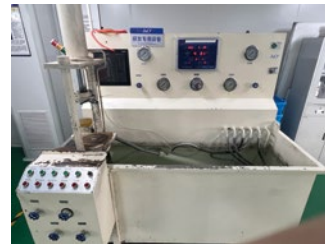
Pressure Test for Large Valve
